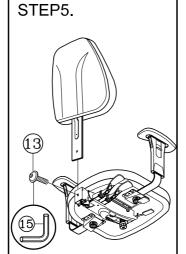
Step 5. Insert backrest post into rear of mechanism and secure using one back bolt (13).
