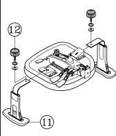
Insert armrests (11) into the brackets located at both sides of the seat.
