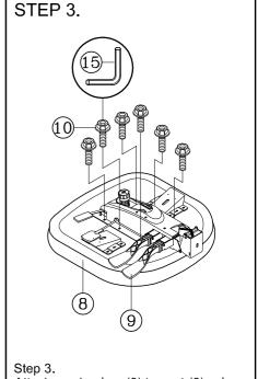
Step 3. Attach mechanism (9) to seat (8) using screws (10).
