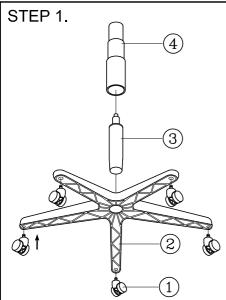
Step 1. Insert the castors (1) into the hole at the bottom of the five prong base (2). Insert the bottom end of the seat post (3) into center hole of the base. Slide seat post cover (4) over seat post.
