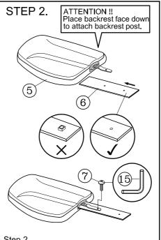
Step 2. Attach backrest post (6) to back (5) using one short backrest post screw (7).
