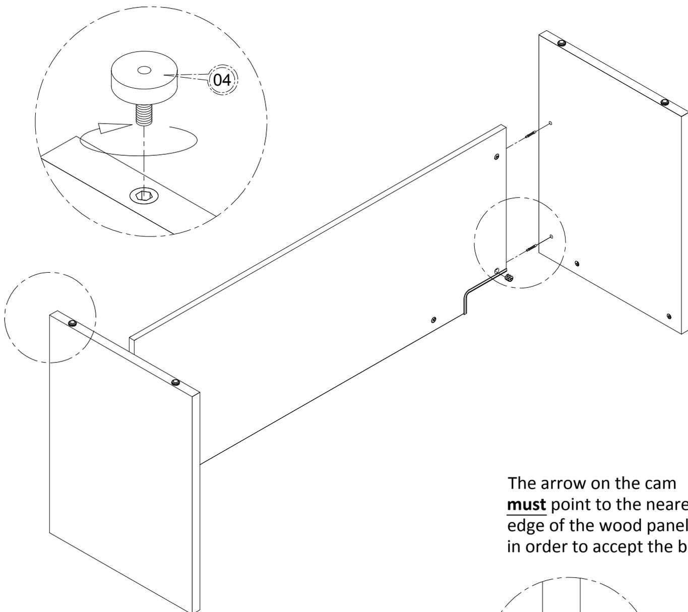
The arrow on the cam **must** point to the nearest edge of the wood panel, in order to accept the bolt
