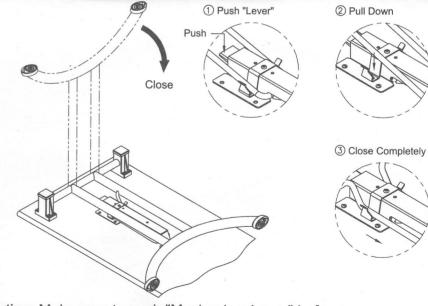
★ Caution: Make sure to push "Mechanism Lever" before pulling down the frame to closed flat position.
