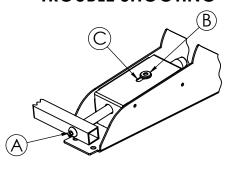
WHEN BOLT "A" IS TIGHTENED DURING ASSEMBLY IT MAY CAUSE THE PLUNGER TO ROTATE CLOCKWISE.
