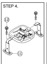
Insert armrests (11) into the brackets located at both sides of the seat.
