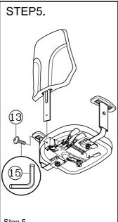
Step 5. Insert backrest post into rear of mechanism and secure using one back bolt (13).
