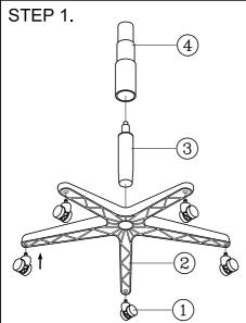
Step 1. Insert the castors (1) into the hole at the bottom of the five prong base (2). Insert the bottom end of the seat post (3) into center hole of the base. Slide seat post cover (4) over seat post.
